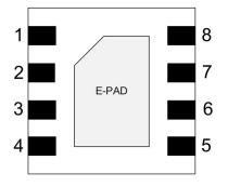
2.0mm x 2.0mm 8 Pin DFN Top View
