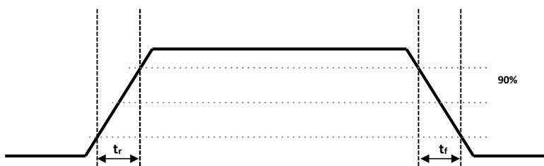
Figure 8. Turn On Rise Time and Turn Off Fall Time
